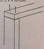
2. Cut four 37-inch lengths of hardware cloth. Fold back the edges of the wire 1 inch. Stretch the pieces of hardware cloth across each frame. Make sure the corners of each frame are square and then staple the screen tightly into place every 4 inches around the edge. The wood and wire frames will be dividers in your composter.
